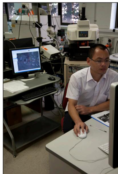
*The Laser-ablation ICPMS microprobe.*
