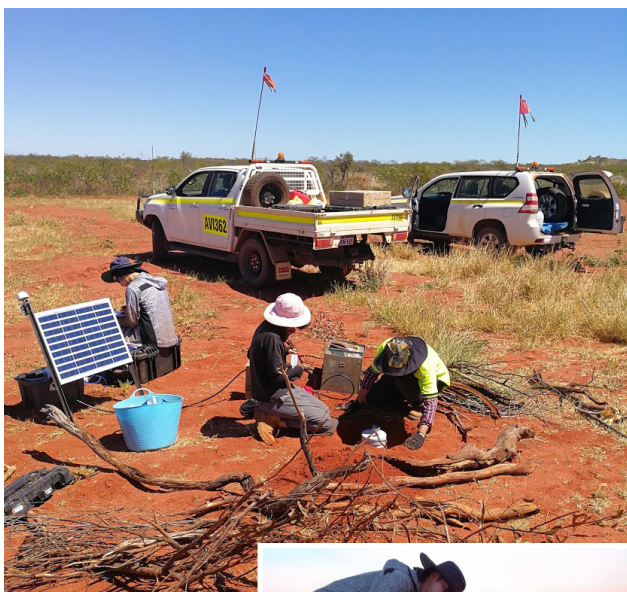
IGG CAS students Chao Lu, Liz Li and visitor Xiangdong Lin installing a temporary seismic station near Pardoo Roadhouse.
