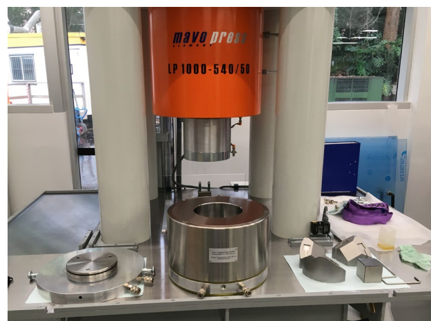
Figure 2. 1000-ton multi-anvil apparatus from Voggenreiter GmbH.
