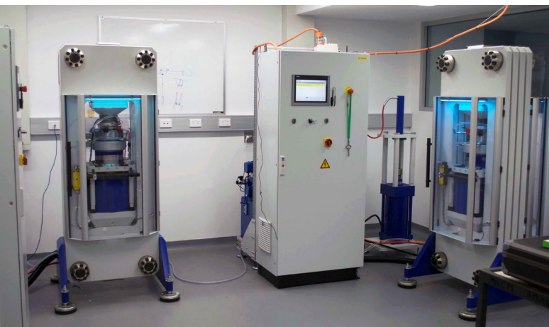
Figure 3. Two new piston-cylinder apparatuses from GUKO Sondermaschinenbau GmbH, installed in January 2020.
