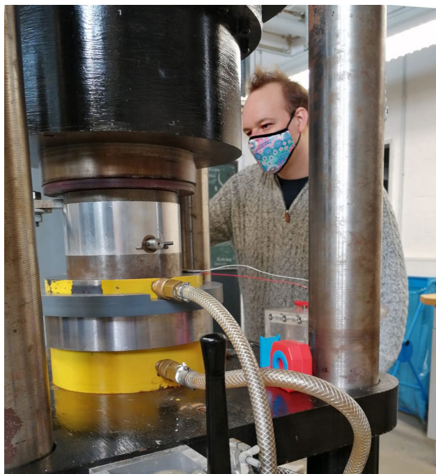
Anthony running a Mica-Pyroxenite melting experiment with the Yellow piston-cylinder as part of his DAAD funded cotutelle with the Institut für Mineralogie, Westfälische Wilhelms-Universität Münster (Photo: Paul Pangritzfor).
